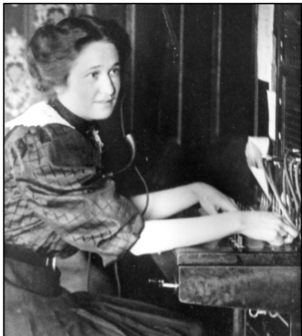
1905 – Telephone communication came to North Ogden. Switchboard operators connected each phone call manually by inserting a pair of phone plugs into the appropriate jacks on an exchange board.
