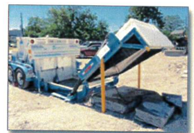
Figure 17. Delivering hardened concrete to a recycler
