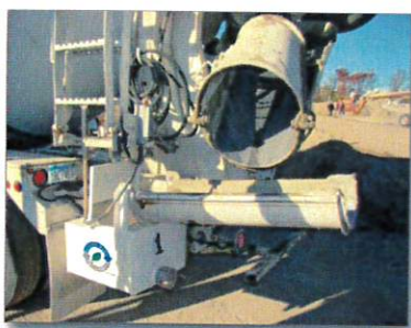
Figure 7. Chute washout box
