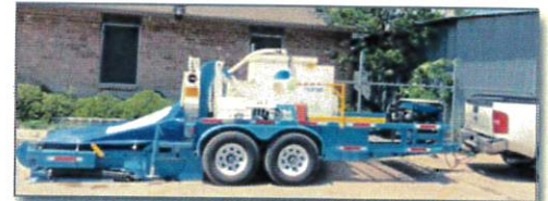
Figure 16. Washout container with a rain cover and onsite washwater treatment
