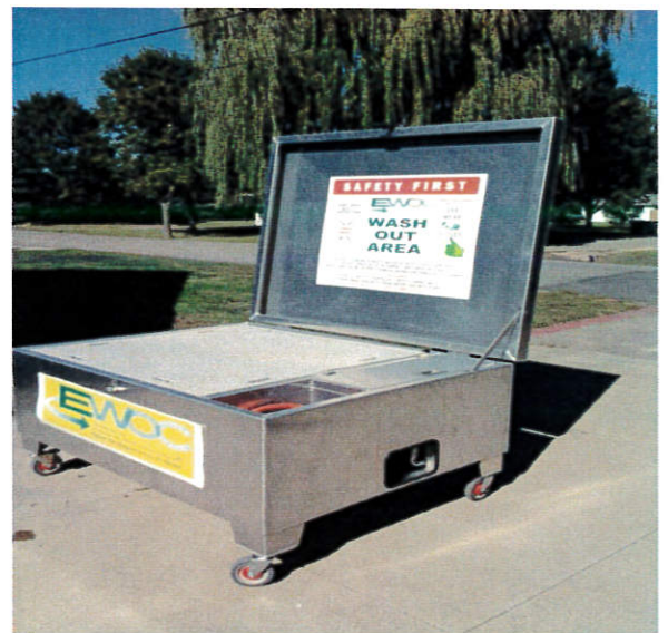
Self-contained washout facility
